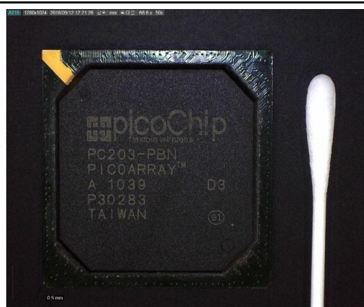
Revision D3 - After Solvent Test for Marking Permanency
