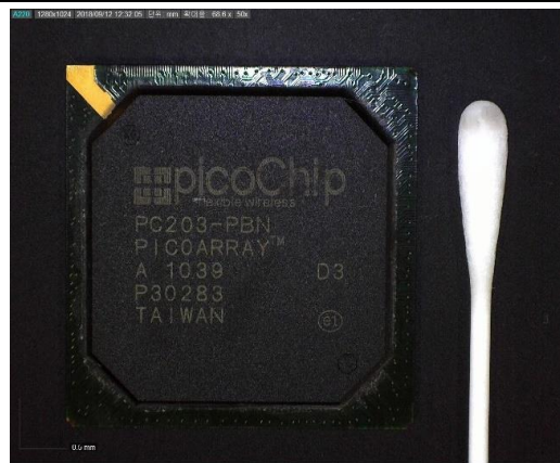
Revision D3 - After Solvent Test for Resurfacing
