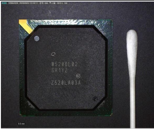
Original Sample - After Solvent Test for Resurfacing
